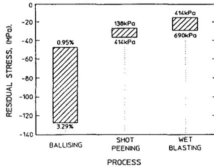
Fig. 9 Comparison of residual stress induced by fatigue life enhancement processes.
