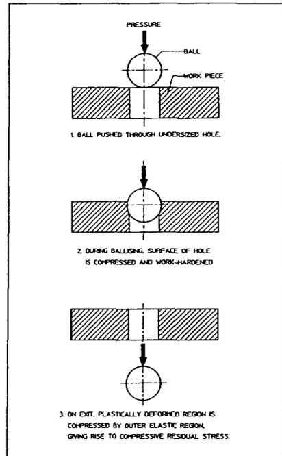
Fig. 1 The ballising process.
