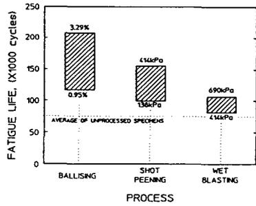
Fig. 7 Comparison of fatigue lives from the three processes used.
