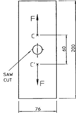
Fig. 4 Specimen for residual stress measurement.
