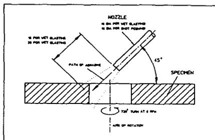
Fig. 3 Setup of the wet blasting process.
