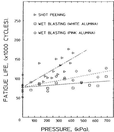
Fig. 5 Fatigue lives of shot peened and wet blasted holes.
