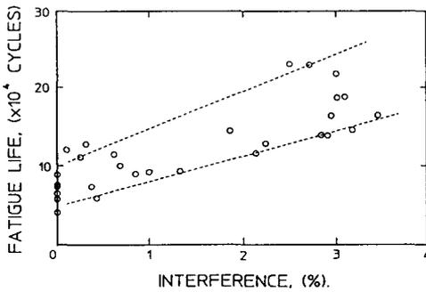
Fig. 6 Fatigue lives of ballised holes.
