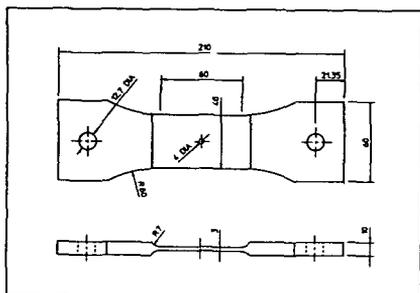
Fig. 2 Dimensions of tensile fatigue test specimen.
