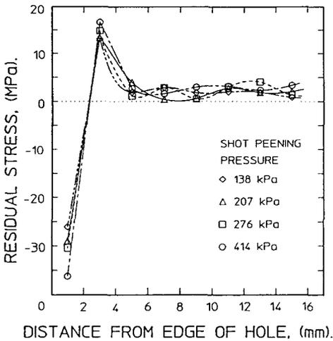
Fig. 8 Residual stress distribution around a shot peened hole.
